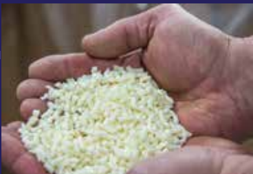
DAVE IS HOLDING A PLASTIC MODIFIER IN THE FORM OF AN EXTRUDED PELLET. THIS MATERIAL IN FINAL FORM WAS PROCESSED INTO A 30 MESH POWDER, OR TWO HUNDREDTHS OF AN INCH.
